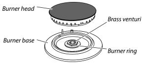
Undo the large brass nuts and remove the brass venturis and brass rings.
